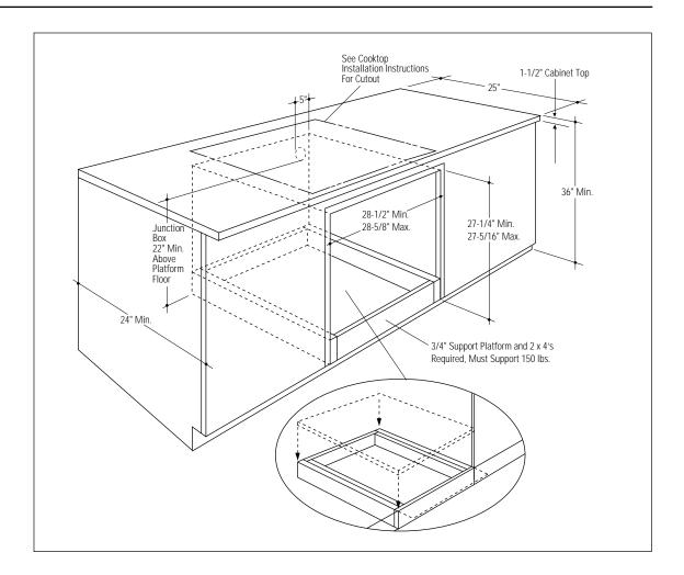
These ovens can be installed below a countertop. The rough opening of the base cabinet should be:
